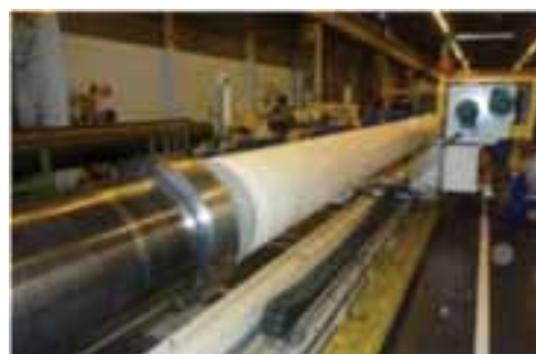
Figure 6—Manufacturing process of the inner composite hose prototype
