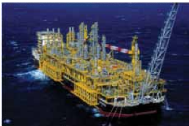
Belanak Natuna Full field production with gas treatment and cryogenic processing. Courtesy of ConocoPhillips
